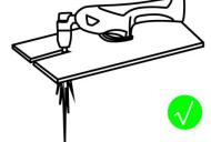
When cutting, select the appropriate current and pushing speed according to the material and thickness of the workpiece to ensure that the spark are exiting from the bottom of the workpiece
