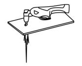
Pull the trigger to start the arc ,The cutting arc will initiate when the torch tip is close enough to the work Piece. Start cutting on the edge until the Arc has cut completely through.
